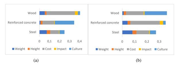
Best alternative and criteria importance to beams of 4 m (a) e 8 m (b) to concrete C50
