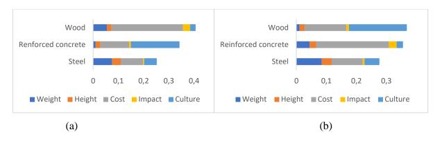
Despite the importance of the cultural criterion, and the fact that wood was the last option in this regard, the wooden beam proved to be preferable among the beams with a 4m span, with a 40.62% priority. This fact is mainly explained by the low cost of this material. For the 8m spans, the reinforced concrete beam was the preferred one with 36.84% of priority, with great influence on the cultural criterion.
