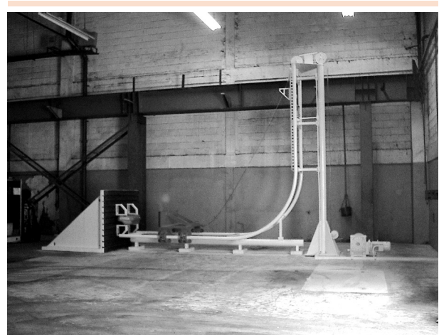
Figure 1: Picture of the sled crash test equipment
