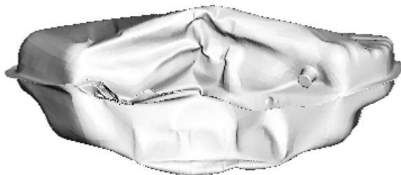
Figure 3: (a) Picture of crashed tank; (b) scanned tank by 3D laser scanner; (c) IGES surface of scanned tank generated by Geomagic software
