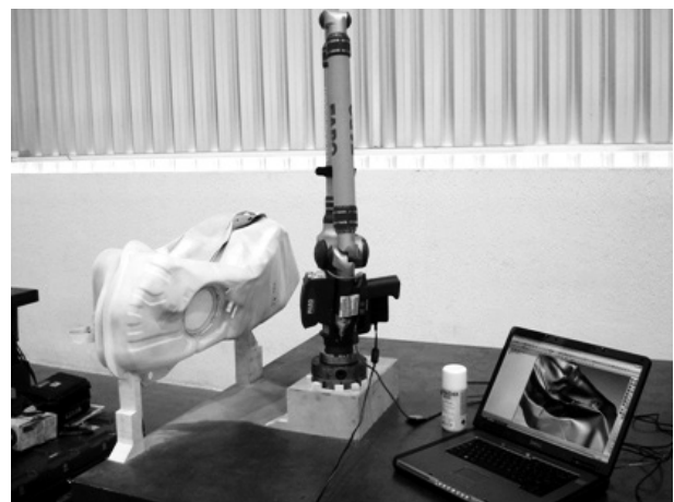
Figure 2: Crashed tank and arm-mounted laser scanner
