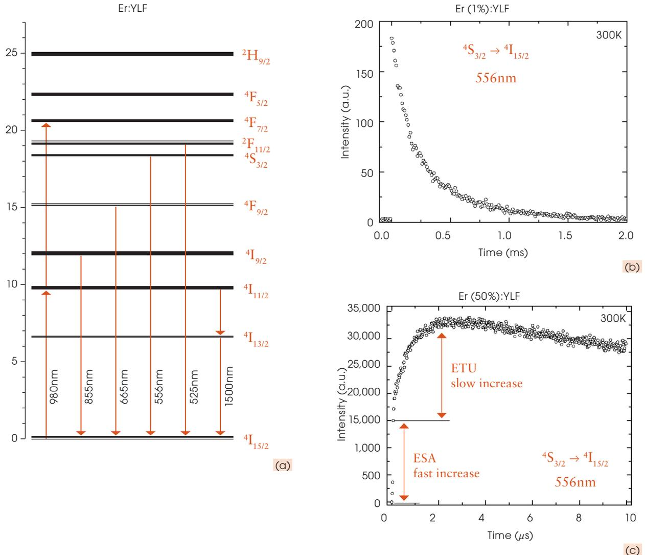
**Graphic 2: (a) Diagram of the energy levels of  $Er^{3+}$  showing all the up-conversion luminescence processes involved; (b) Luminescence decay curve of the 556 nm emission for the Er (1 mol%) that occurs by ESA process; (c) Luminescence decay curve of the 556 nm emission in the Er (50 mol%) obtained by ESA and ETU**
