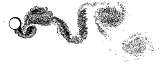
**Figure 5: Cylinder in its lowest position ( $t = 15$ , when  $\omega = 1.5$  and  $A = 0.5$ )**
