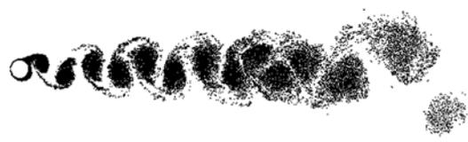
**Figure 4: Wake pattern when the body oscillates with small amplitude and low frequency,  $Re = 10^5$**
