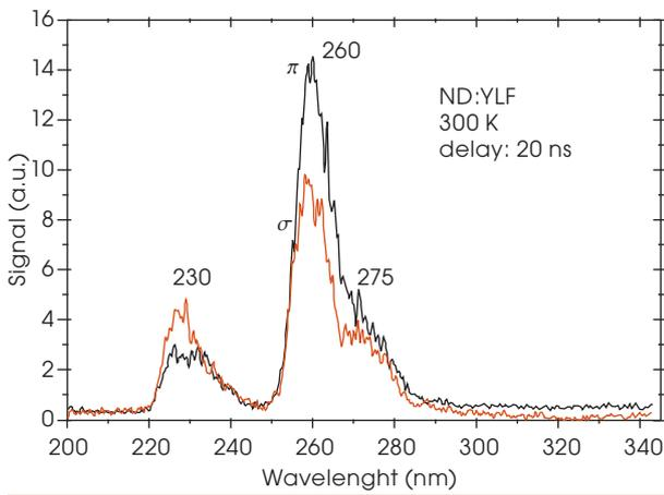
**Graphic 2: Polarized emission spectrum of the  $4f^2 5d$  configuration of Nd:YLF crystals, after three photons absorptions of 532 nm**
