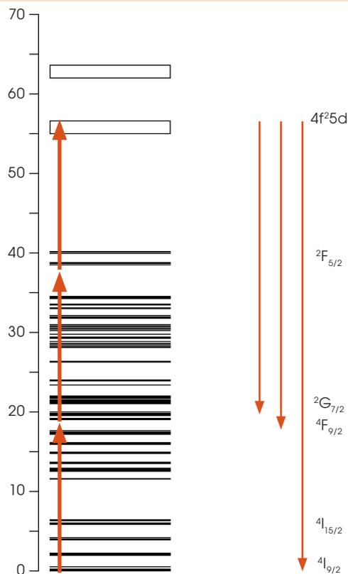
**Graphic 1: Energy level diagram of Nd:YLF showing the three-photon excitation scheme and the observed transitions from decay of the  $4f^25d$  configuration<sup>2</sup> (1 nm= 250 cm<sup>-1</sup>)**
