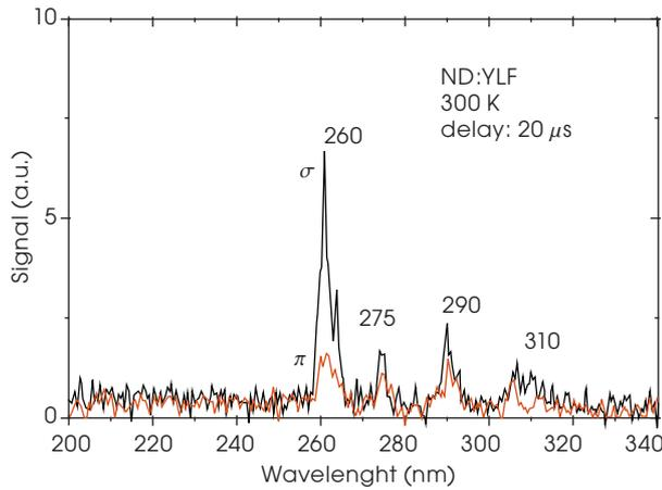
**Graphic 3: Polarized emission spectrum of the  $4f^3$  configuration after two photons absorption of 532 nm in Nd:YLF crystal**
