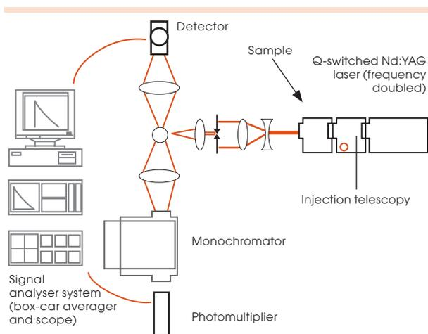
**Illustration 1: Experimental setup for luminescence measurements**
