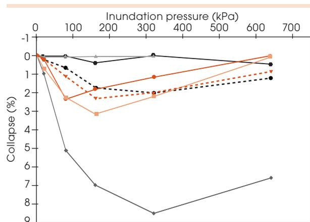
**Graphic 1: Curves of collapse of the soil for some depths**
