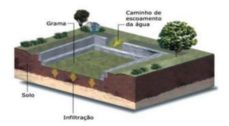
Figure 8 - Example of a rainwater retention zone.
