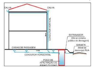
Figure 9 - Schematic detail of the rainwater infiltration system model
