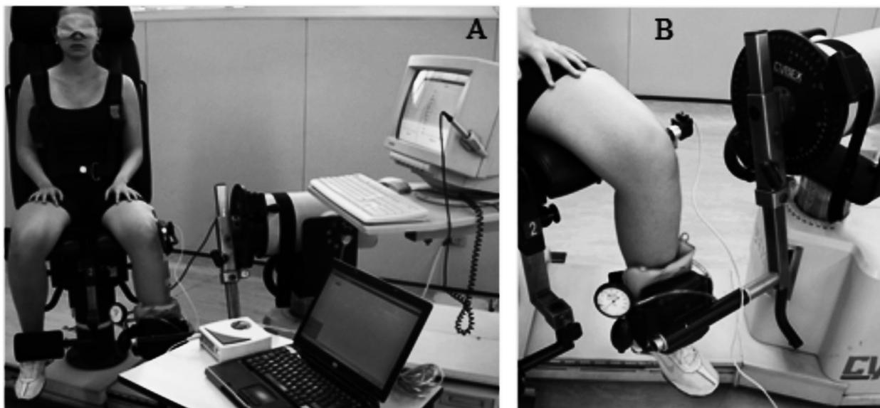
**Figure 1:** A – Open kinetic chain exercises position; B – Detailed position of the sphygmomanometer and electrogoniometer
